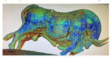
defining a surface, to be derived from points within two 2D pictures that have been taken from slightly different positions. In this case, the points within each of the 2D pictures (i.e., the points known to be the same in the two pictures) were determined by the intersection of horizontal and vertical laser lines that were scanned across
