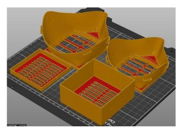
While slicing software is designed primarily to convert object models into instructions for a 3D printer, they often have other noteworthy features. Most slicing software, for instance, allows you to control the infill. Other types of slicing software allow you to add supporting structures, which are oftentimes essential large and complex for objects. Furthermore, rafts, skirts and brims can all be controlled in slicing software.
